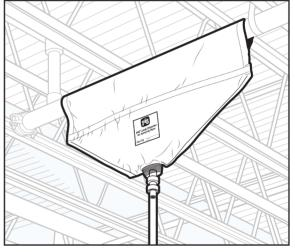
4. Make sure unit is centered on the leak and position hose in drain receptacle or collection container.
