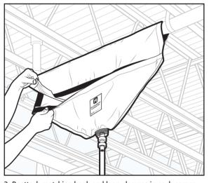
3. Reattach matching hook and loop closures in each corner, then reattach all other closures until unit fits snug to pipe.
