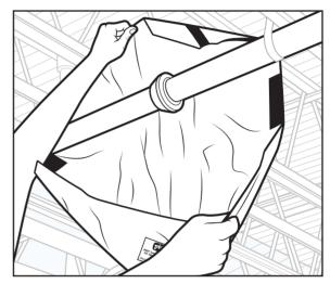
2. Pull the hook and loop fasteners apart and wrap unit over the top of the leaking pipe area. Make sure the attached hose is on the bottom, facing down.
